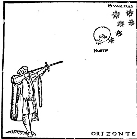
6. Explorers used an astrolabe or cross-staff (shown here) to determine latitude by "shooting" the angle of the sun or the north star at its zenith in relation to the horizon, then reading from a table that listed latitude entries for that angle for every day of the year. Juan de Escalante de Mendoza, Itinerario de navegación de los mares y tierras occidentales (1575). Courtesy, Jerald Milanich.
